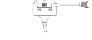
➤ The fuse is inside the *rewireable plug*. Use a screwdriver to remove the plug's back cover. *Never put the plug into the mains socket when its cover is removed*. Lever out the fuse and replace it with a new one. Replace the plug's back cover.
