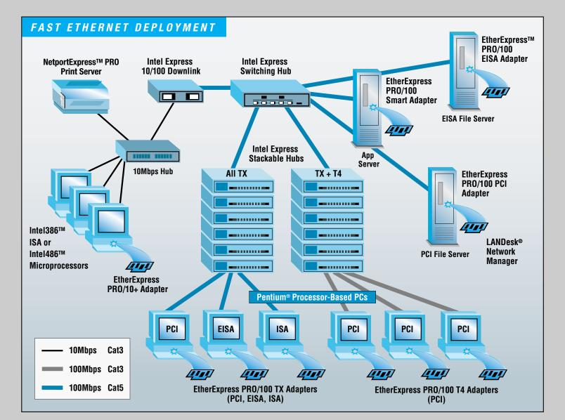
Today's high performance operating systems and bandwidth-hungry applications like CAD/CAM, multimedia or the Internet can cause data bottlenecks that slow workgroup performance. With Intel's Fast Ethernet family of products, you can easily unplug those bottlenecks by making the move to high speed networking. Future-proof your Pentium<sup>®</sup> processor-based machines with EtherExpress™ PRO/100 Adapters, then go to 100Mbps on an "as-needed" basis using Intel Fast Ethernet products.
