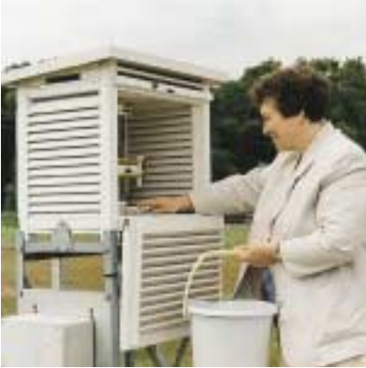
A few additional tasks, such as cleaning the thermometer screen, are required periodically
