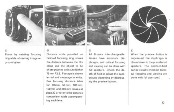
5. Focus by rotating focusing ring while observing image on ground glass.
