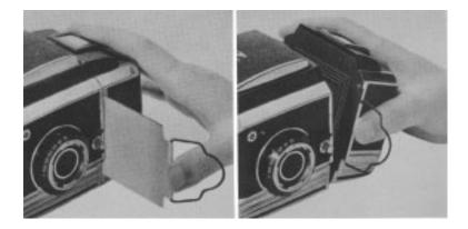
The standard Bronica S2A film back magazine is specially designed to accept either the 12 exposure 120 or the 24 exposure 220 roll film. With the Model-E film back magazine, you can get 16 (6x4.5) exposures on the 120 film and 32 (6x4.5) exposures on the 220 film.
