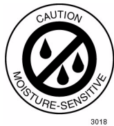
Figure 12.5 A moisture-sensitive ID label is applied to the outside of the box in which the dry-packed parts are packed.
