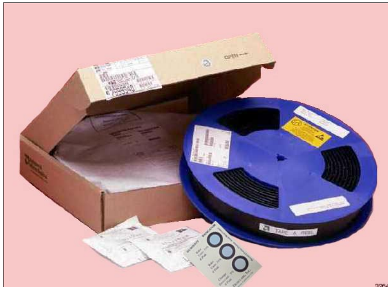
Figure 12.1 Moisture-sensitive product is first baked to remove excess moisture and then packed in a dry pack bag (shown in the box) with desiccant and a humidity indicator card.
