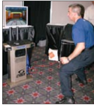
Paul Dolan demonstrates the CYBEX Trazer, a reaction trainer using an interactive virtual world to improve muscle and mental agility. Reaction time, acceleration, speed, power and balance drive the user’s on-screen activities.
