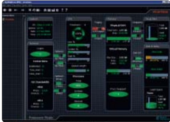
Quest's Spotlight for both Windows and Unix gives you a dashboard view of the critical metrics for server health. Here, Spotlight highlights a problem with our Linux server under testing, with paging and unusual disk activity.
