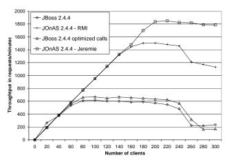
Figure 11. DAO separation EB CMP throughput in interactions per minute as a function of number of clients for the bidding mix using JBoss and JOnAS.
