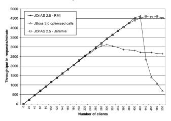
Figure 18. EJB 2.0 local interfaces implementation throughput in interactions per minute as a function of number of clients for the browsing mix using JBoss and JOnAS.
