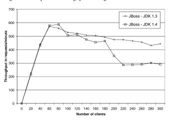
Figure 22. EB CMP implementation throughput in interactions per minute as a function of number of clients for the browsing mix using JBoss 2.4.4 for JDK 1.3 and 1.4.
