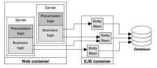
Figure 3. DAO separation with Entity Beans.
