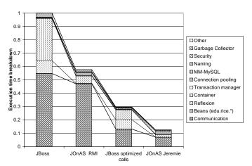
Figure 17. Execution time breakdown for the session façade implementation for the bidding mix at the peak point of the *JBoss* configuration.
