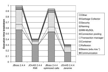
Figure 14. Execution time breakdown for the EB BMP implementation for the bidding mix at the peak point of the *JBoss* configuration.
