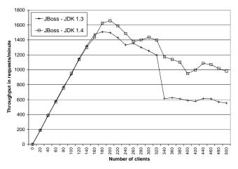
Figure 26. Session façade implementation throughput in interactions per minute as a function of number of clients for the bidding mix using JBoss 2.4.4 using JDK 1.3 and 1.4.
