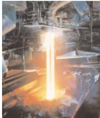
Filling bottle moulds with molten glass
