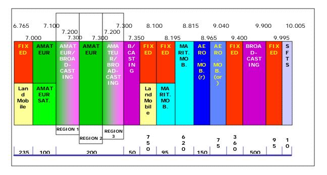
In the Diagram 2 above, its shown that some of the spectrum was allocated to a single service (exclusive allocation) and some are allocated to more than 1 service (sharing allocation). Further more, each service was allocated with a different bandwidth. Details are as in the Table 2 below.
