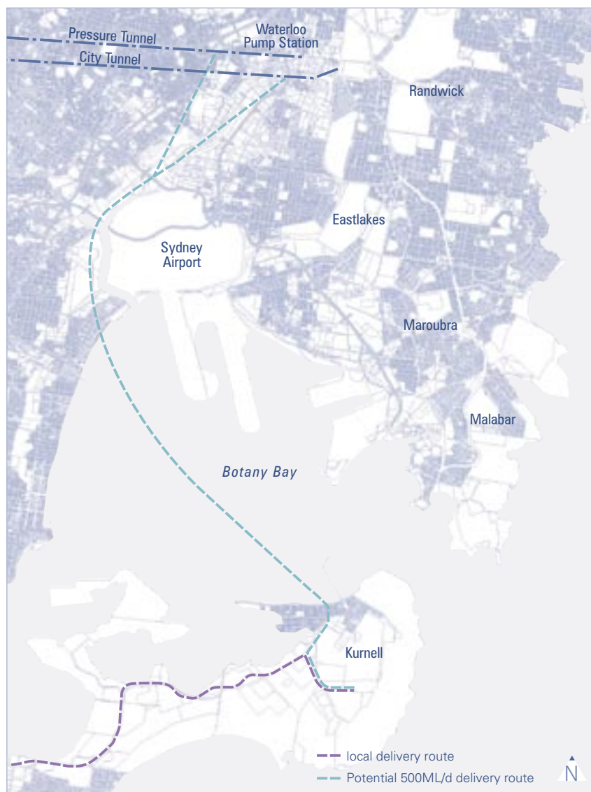
Figure 7.2 One Potential Water Distribution Route for a 500ML/day Desalination Plant at Kurnell
