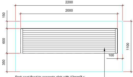
Park seat fixed to concrete slab with 12mmØ x 100mm long Dyna bolts. Tightly fix dome nut to protrubing thread above fixing nut. Dome nut shall firmly butt against top of fixing nut. Ensure nuts are tamper proof.
